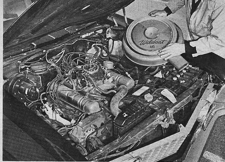
Big 401 produces 325 hp at 4400 rpm and hefty 445 lb/ft of torque at 2800 rpm.
